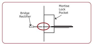
6 Carefully slip the connected mortise lock chassis into the mortise pocket paying close attention not to pinch any wires.
