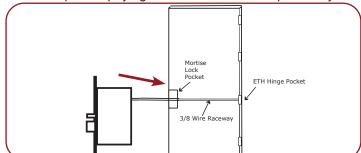
Connect the wires from the power supply at the ETH hinge on the jamb side. Connect the hinge to the jamb.
