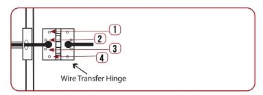
**5** Connect the Bridge Rectifier to the plug exiting the mortise chassis.
