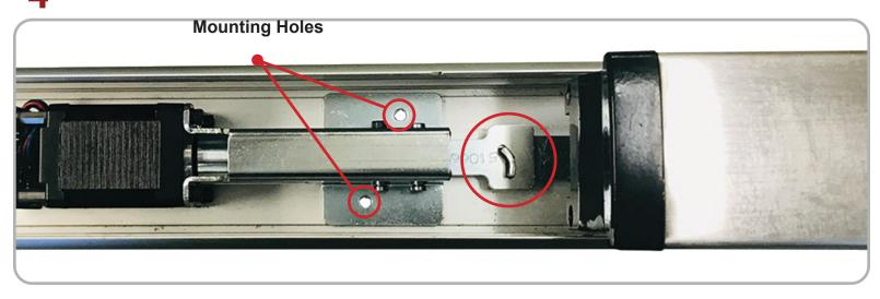
With one hand holding the motor in place, flip the bar over and secure the kit by installing the two provided screws into the **Mounting Holes** from the backside of the bar.
