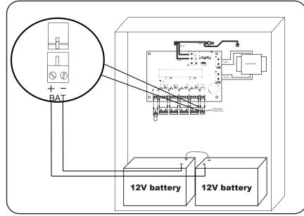
Fig. 3.2 - Wiring off 1 relay
