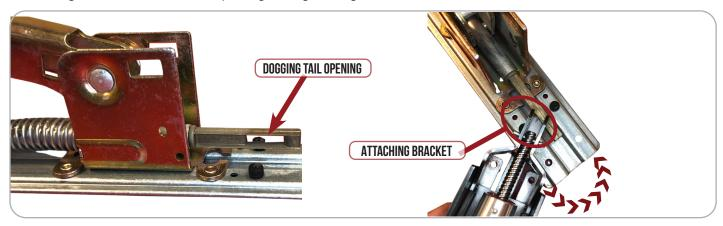
**Straighten Motor kit**, depress the back activating bracket & gently pull back on the motor kit to slide the mounting bracket **UNDERNEATH** the baserail.
