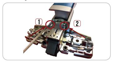
**3.** Slide off (1) Housing to expose Pushpad & Baserail Assembly. Next, (2) remove push pad.
