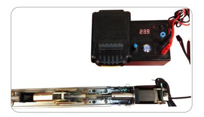
**11.** Re-install Push Pad (1), then slide the exit device housing back onto the device (2).
