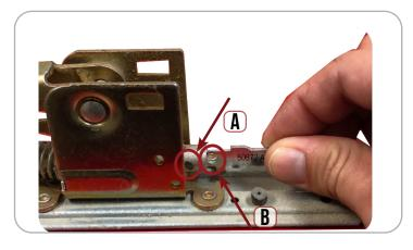
**6.** Line up Holes A & B, insert pin & secure it with the clip provided. If you have an older device without Hole B, please scan the QR code for a video how to use the provided dogging kit.
