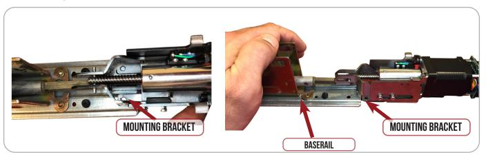
**9.** Line up mounting bracket holes with existing holes on baserail. **Secure Motor kit** to baserail by installing (2) screws provided from the top of the device, not from underneath.
