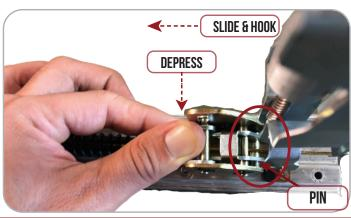
6. Once hooked onto PIN, bring the motor down & slid the mounting bracket underneath the baserail.
