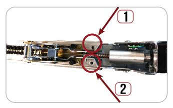
9. Replace mounting bracket & Re-install (2) screws.
