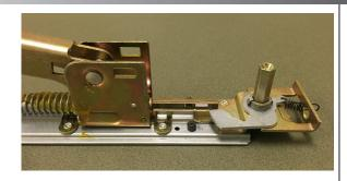
2. Drill top hole with 9/64 drill bit provided.
