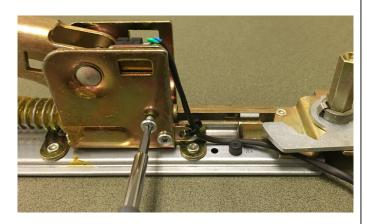
5. Test switch for correct operation.
