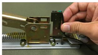
4. Use the screws provided and secure the kit to the bracket.
