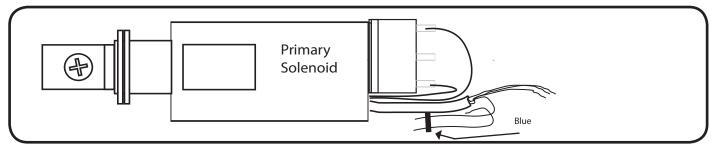
C. Connect White and Red wires from solenoid to RED wire from harness. Next, connect Black wire from solenoid to BLACK wire from harness. Next, connect PM300.
