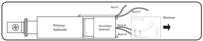
B. Connect Red #1 solenoid wire to RED harness wire. Next, connect Black #1 to BLACK harness wire. Disregard the two Secondary Black wires. Next, connect PM300.
